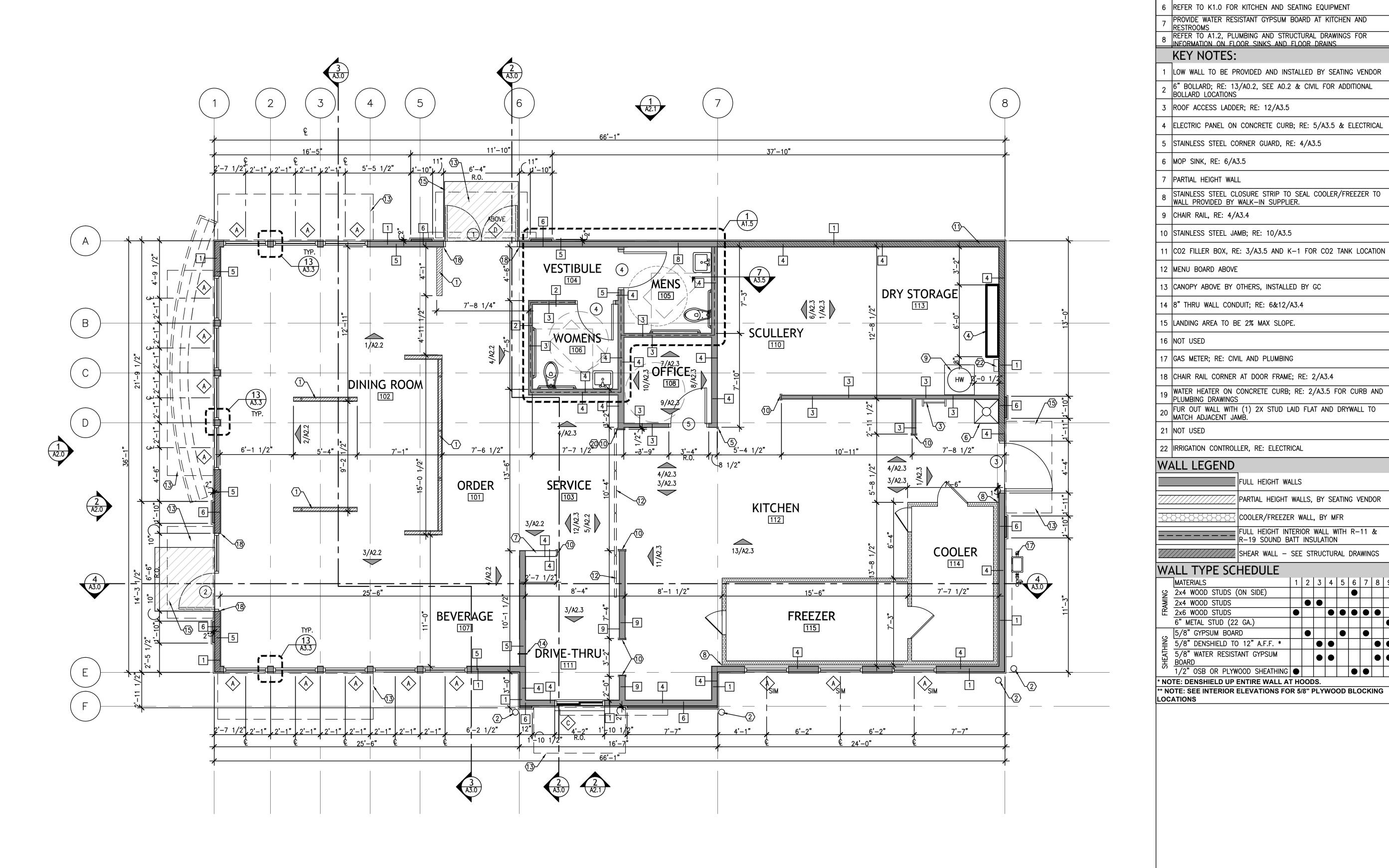
**GENERAL NOTES** ALL INTERIOR DIMENSIONS ARE SHOWN TO FACE OF FRAMING UNLESS NOTED OTHERWISE. EXTERIOR WALLS ARE DIMENSIONED TO FACE OF STEM WALL/FACE OF SHEATHING. OPENINGS ARE DIMENSIONED TO FACE OF FRAMING. B EXTERIOR SHEATHING TO ALIGN WITH FACE OF STEM WALL. 4 REFER TO FINISH SCHEDULE SHEET A4.0 FOR APPLIED FINISHES.
